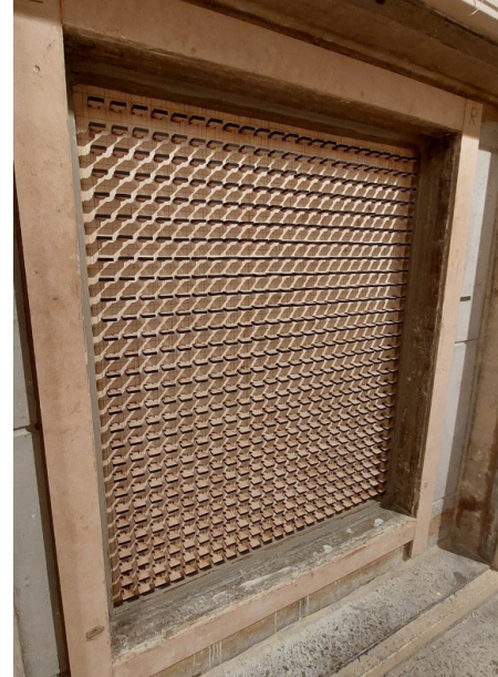
Figure 3: Fabricated multi-modal metamaterial panel, mounted in the transmission opening of the Laboratory of Acoustics of KU Leuven.
