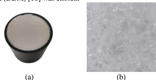
Figure 3. Melamine samples (a) and details of the melamine porous material (b)
