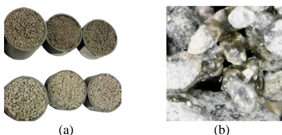
Figure 2. Porous concrete samples (a) and details of the porous concrete material (b)
