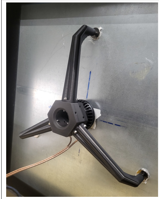
Figure 2. Prototype of the actuator attached to the steel metal plate in the test rig.
