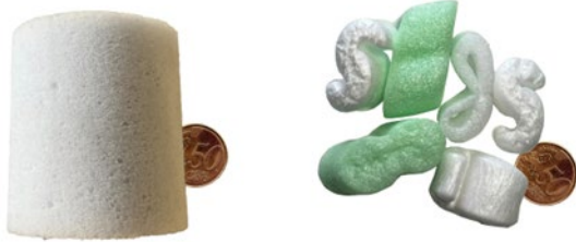
Figure 2. Detailed view of investigated materials: Left: melamine foam (cylinder cut out of the 50mm thick panel). Right: Selection of flo-pak granules from the 50 mm loose stack
