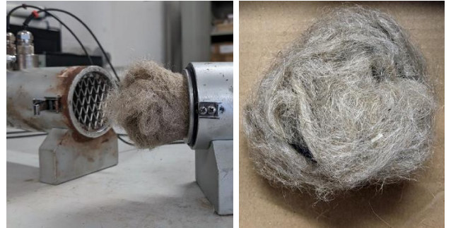
Figure 1. Loose jute fibers and their installation in the plane wave impedance tube.
