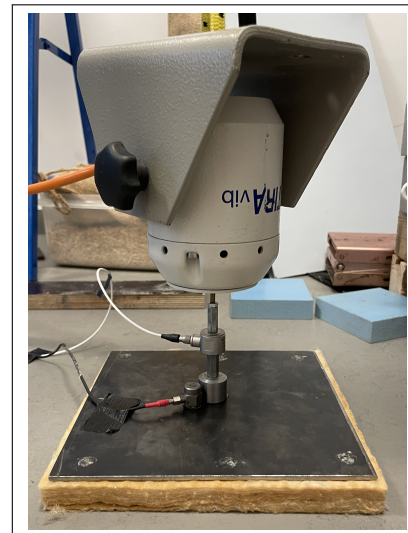
Figure 1. Example of a measurement setup - measurement of a sample marked Light MW.
