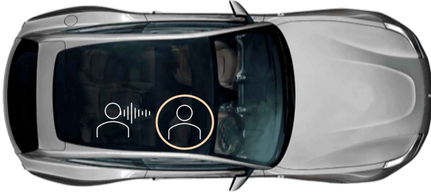
Figure 1. Measurement setup. Speaker at the rear-right seat and listener at the front-right seat along with the ARNC system.
