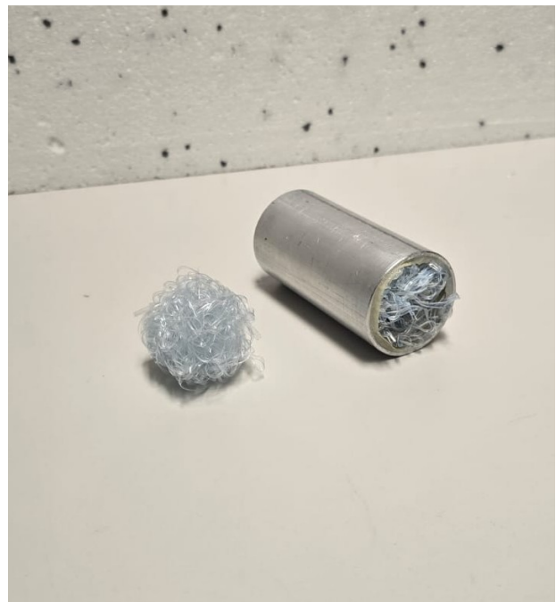
Figure 2. Example of a sample after thermal treatment and a 100 mm sample ready to be tested in the impedance tube.
