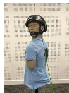
Figure 3. The SECT affixed to a helmet and connected to earplugs.
