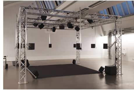
Figure 3. Ambisonic playback system in Mixed-Reality-Lab of Berlin University of the Arts used for the listening experiment. Source: https://berlin-open-lab.org
