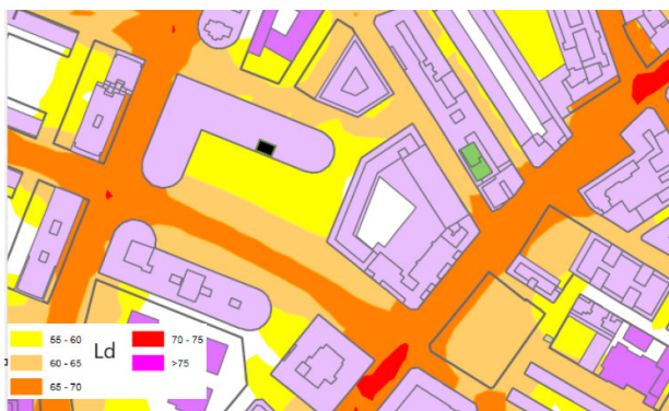
Figure 2. Example of measurement point (in black) and acoustic mapping of the area.
