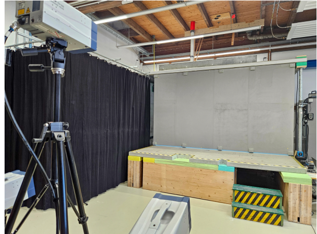
Figure 1: Test Rig showing the 15 mm perspex reception plate coated with a highly reflective surface layer (silver-grey) in combination with a 3D Laser Scanning Vibrometer.
