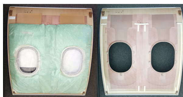
Figure 1. Lining panel; left: condition as supplied; right: test condition.
