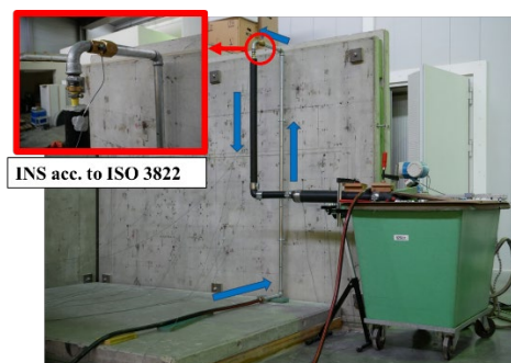
Figure 1. Short pipe section from previous investigations on the reception plate [5,6], the same pipe system is investigated in the installation test stand. Blue arrows depict the water flow direction.
