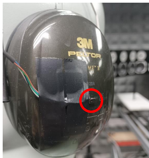
Figure 1. MEMS microphone placed in the earmuff of the hearing protection headset.
