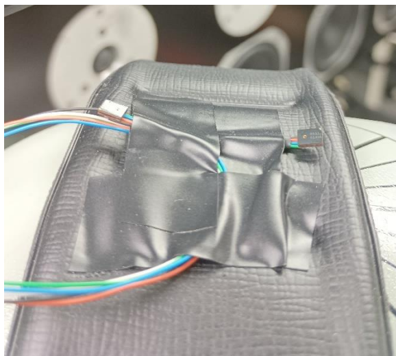
Figure 2. MEMS microphones placed on the headband of the hearing protection headset
