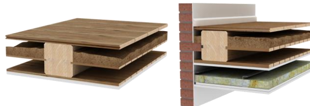
Figure 4. Timber floor constructions. The left drawing shows the original construction, the drawing to the right includes a new self-supporting ceiling. The drawings are from https://gi.dk/byggeteknisk-viden/ .
