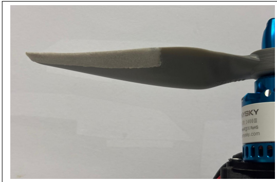
Figure 1. Propeller APC 8X6 E with a roughness value of 50 \mu\text{m}
