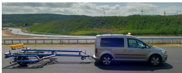
Figure 1. Open CPX trailer used for measurements (designed by CDV).
