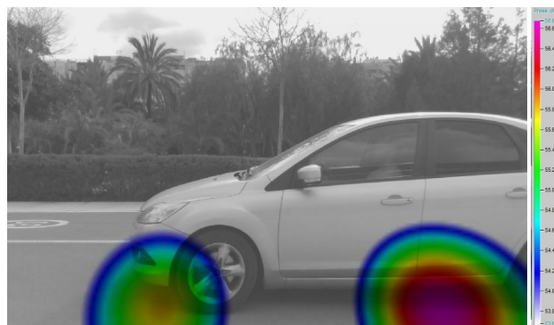
Figure 4. 1 KHz band SPL (dB), conventional surface
