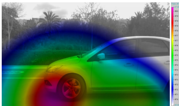
Figure 2. Broad band SPL (dB), conventional surface
