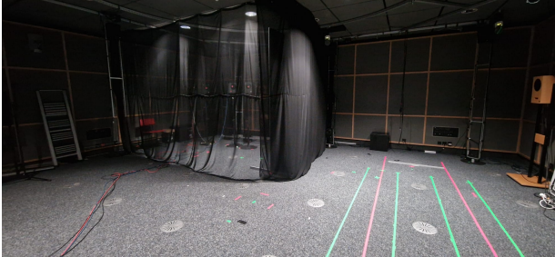
Figure 1: Overview of the test setup under normal light conditions. The green markings indicate Lines 1 to 4 used in the 'Large-scale Test' and the pink markings indicate Line A and B used in the expert test. Minimal lighting was used during the tests.
