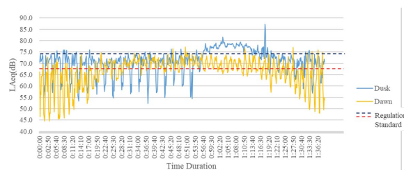
Figure 7. Measured sound pressure levels and residential noise regulation thresholds [11].
