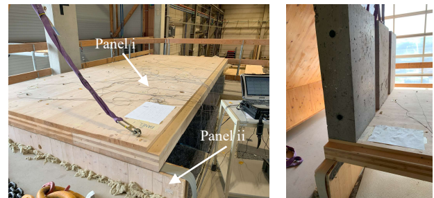
Figure 1. Horizontal L-junction CLT mockup. On the left without extra weight. On the right with three concrete blocks.
