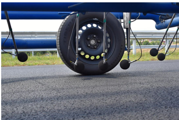
Figure 1. Real locations of the individual measuring microphones around the reference tyre on CPX trailer.
