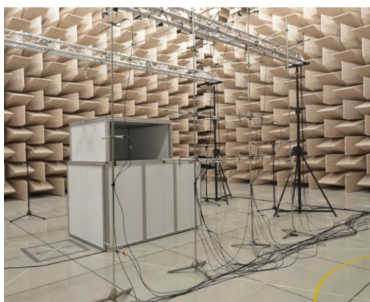
Figure 7. Model machine 1 and 18 additional measurement positions according to ISO 3744 in the hemi-anechoic chamber at BAuA.
