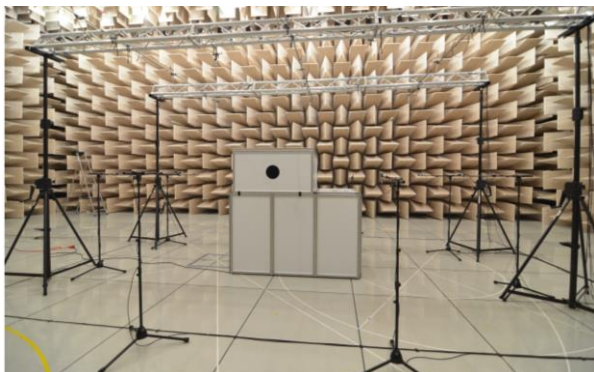
Figure 6. Model machine 1 and the setup according to ISO 3744 in the hemi-anechoic chamber at BAuA.
