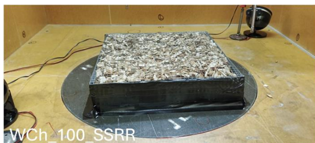
Figure 2. Small-scale reverberation room (SSRR) sound absorption measurements: WCh_100_SSRR.
