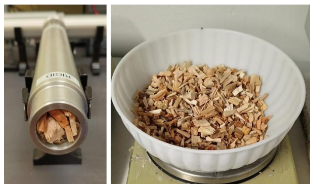
Figure 1. Impedance tube sound absorption measurements: randomly mixed sizes of loose wood chips for samples WCh_20_1-4 and WCh_100_IT.
