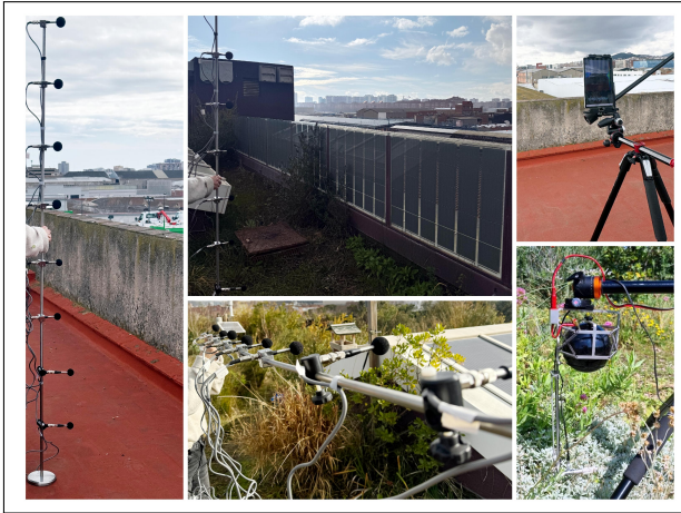
Figure 2: Photo collage of five key scenes. Left: vertical array of microphones in front of a conventional wall parapet. Middle top: vertical array of microphones in front of a photovoltaic glass of width 0.02 m. Middle bottom: horizontal array of microphones along a vegetated zone. Right top: acoustic camera facing a conventional wall parapet. Right bottom: impedance gun measuring absorption of a vegetated surface.
