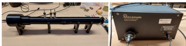
Figure 3. The measurement setup with the impedance tube and data acquisition device.
