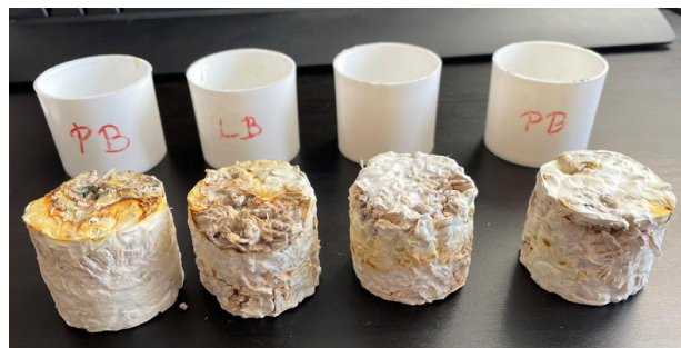
Figure 2. Examples of homemade breeding on beech wood chips substrates using Ganoderma lucidum and Pleurotus in small size for acoustic testing.
