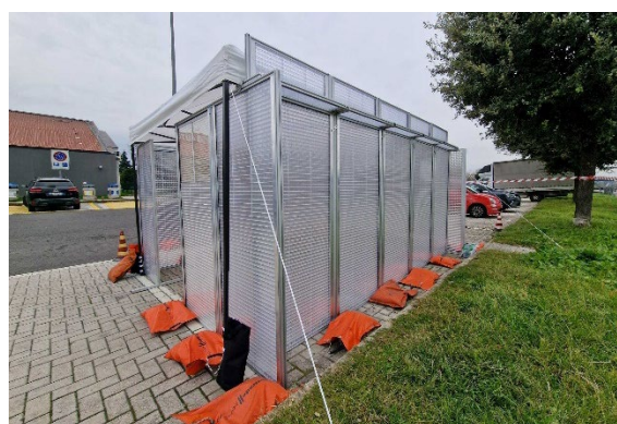
Figure 1. The metamaterial structure used in this study, mounted at the service station Peretola Sud .
