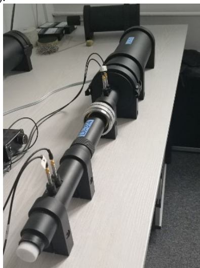
Figure 2. Impedance tube used for measurement of the acoustical parameters
