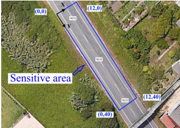
Figure 3: Google Maps® image used for the generation of the homography matrix and the identification of the sensitive area for the vehicles' recognition.
