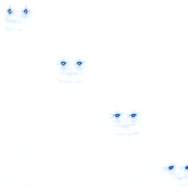
Figure 557. Hardware beamformed TFM with imasonic 128 elements 15MHz center frequency, 0.25 pitch probe, 36x50mm, 256 x 750pixels.
