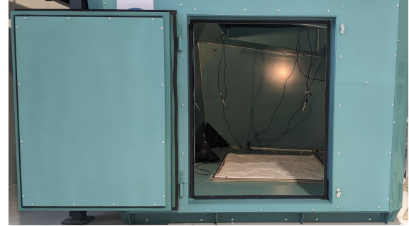
Figure 2: Polyester fiber sound absorption coefficient measures in an Alpha cabin using ISO 354:2003 standard.
