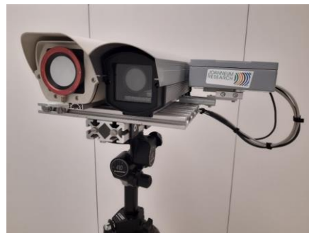
Figure 2. Visual sensors consisting of a synchronized RGB and TIR camera.
