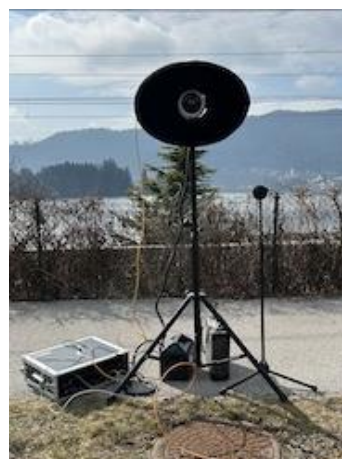
Figure 3. Acoustic sensors including the Class-1 sound level meter and the acoustic camera. The latter consists of a 2D-elliptic, 16 channel microphone array and a 360° camera.
