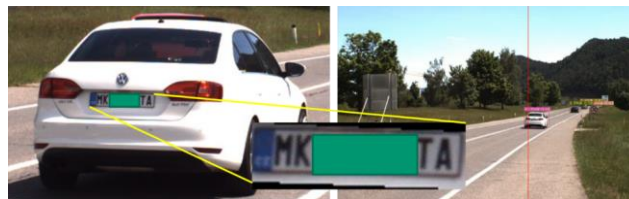
Figure 6. Results from the visual analysis of the sound event from Figure 5. The vehicle is detected in the corresponding RGB frame and identified by the license plate recognition.
