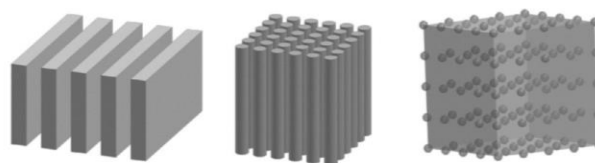
Figure 3: Different types of Sonic Crystals, also known as periodic structures
