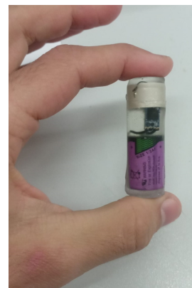
Figure 2. Bidirectional acoustic tag transparent test encapsulation showing i. the piezoelectric element (white cylinder), ii. the electronics (blue board), and iii. the battery (purple cylinder)
