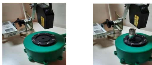
Figure 4. Measurement of the resting point (left), and the displacement with a known mass (right)
