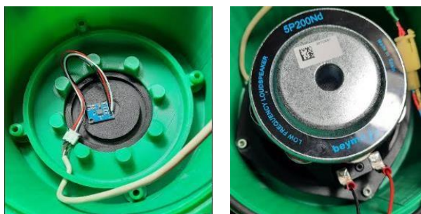
Figure 5. Accelerometer fixed on the back side of the piston (left) with the 5" unit mounted inside the cabinet (right)
