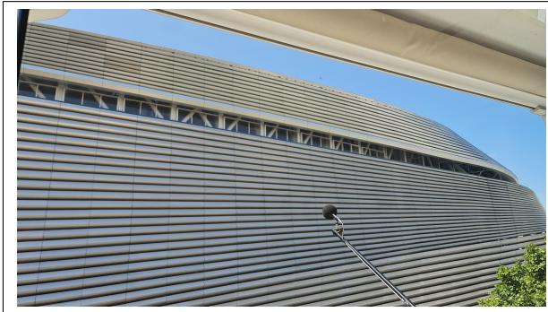
Figure 2. View of the microphone on the façade from a house in the vicinity of the stadium.
