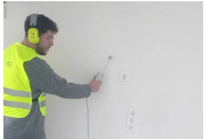
Figure 2. Measurement of incident sound power, scanning the surface approximately at 3 cm of partitions, using Sonocat probe.
