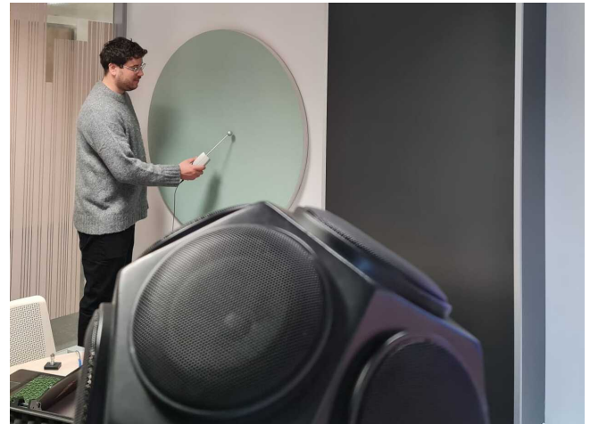
Figure 5. Example of measurement setup of the sound absorption using Sonocat.
