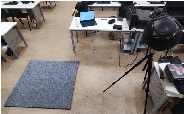
Figure 4. Setup for the measurement of the absorption coefficient with 45° incidence sound.
