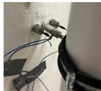
Figure 2: A force transducer and two accelerometers on the installation wall.
