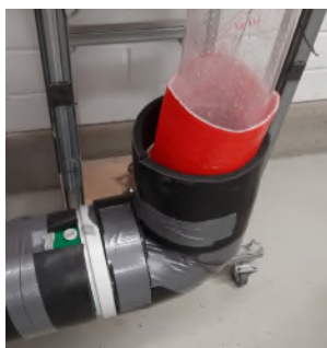
Figure 3: The decoupled basement bend covered by mass-loaded pipe insulation with the loose waterproof membrane cover.
