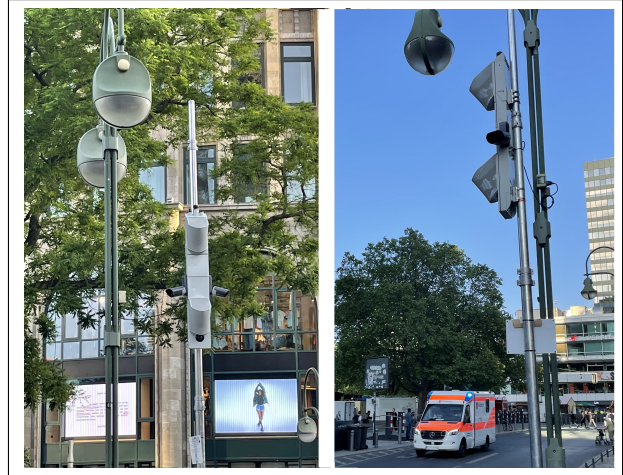
Figure 1. Installed noise radar system Hydre (Bruitparif) at Kurfürstendamm in Berlin, Germany. Photos were taken from two angles by the authors.
