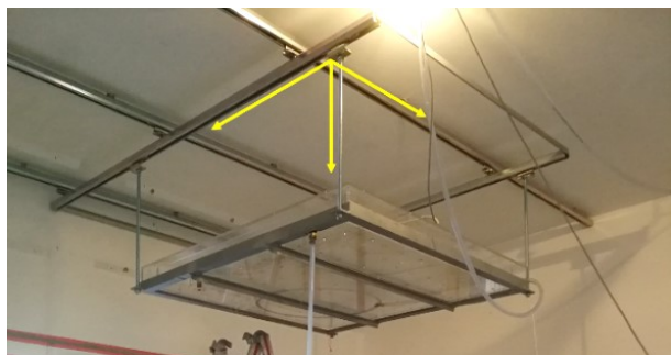
Figure 1. Water tank with perforated bottom to produce artificial rain in a positioning system with guide rails.
