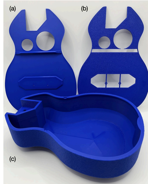
Figure 1. (a) Printed soundboard, (b) Template for constructing the wooden soundboards and (c) 3D-printed resonance box.
