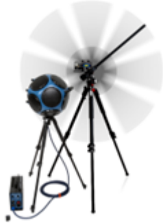
Figure 8. Co-located arrangement of omnidirectional source and rotating linear array.
