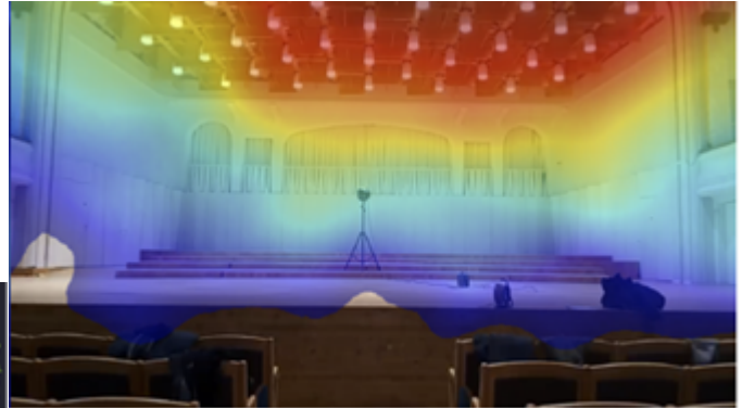
Figure 14. Critical reflections located at the point of observation. Selected frequency band is 250Hz – 3.1kHz at a dynamic range of 6dB.
