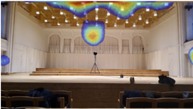
Figure 13. Primary reflections located at the point of observation. Selected frequency band is 250Hz – 3.1kHz at a dynamic range of 2dB.
