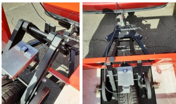
Figure 2. Detail of the laser sensor employed for the rolling resistance tests.
