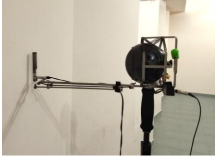
Figure 5. Microflown Technologies impedance gun. Set-up used during measurements for the estimation of the wall absorption coefficient.
