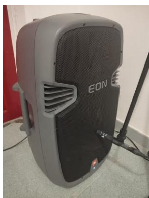
Figure 2. Full-range loudspeaker JBL EON315. Set-up used during on-axis driver measurements.
