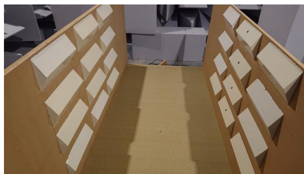
Figure 2. Scale model showing a single configuration of 24 self-shielding façade elements (with 60° outer angles). Four microphones are visible along the right façade centrally positioned in the upwardly directed faces.
