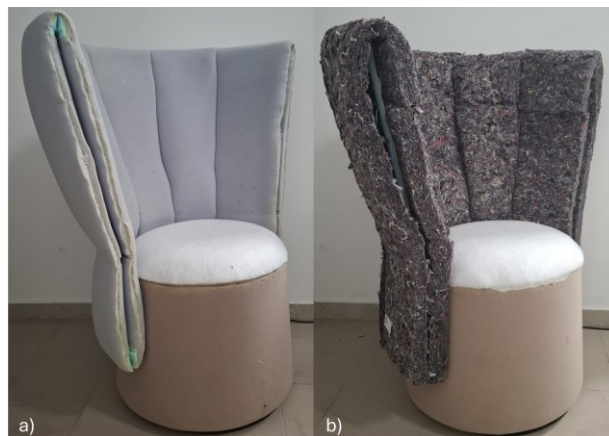
Figure 1. Prototype of the armchair PUR according to the standard design (a) and of the TW one after the padding replacement (b)
