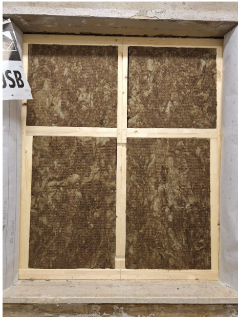
Figure 6. View of the traditional sample with rock wool, before internal finishing.
