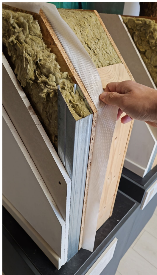
Figure 5. Stratigraphy of the tested walls.
