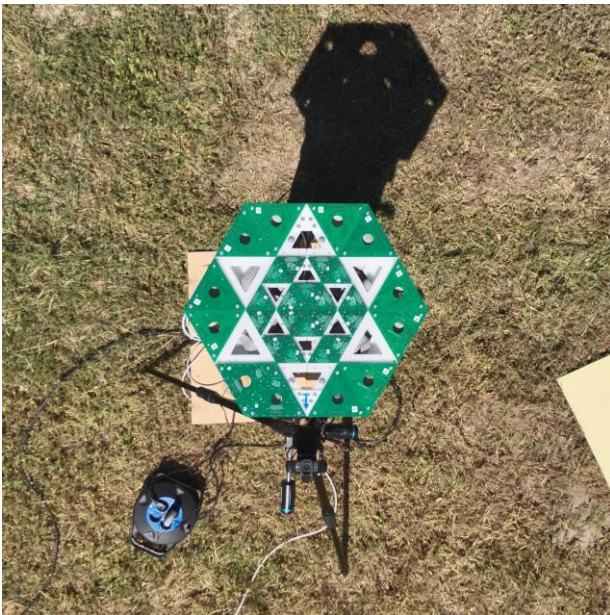
Figure 1. Array of MEMS microphones.
