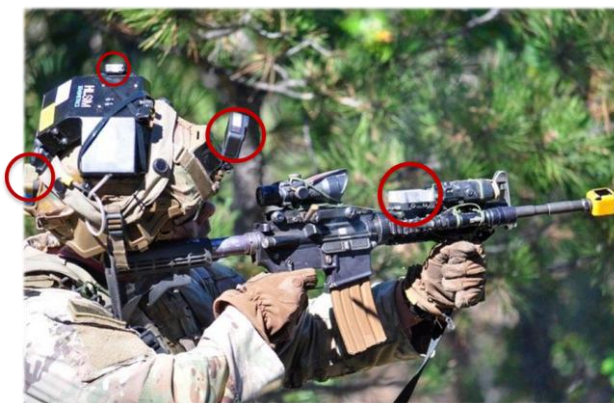
Figure 1. Fully equipped Soldier with red circles highlighting from left to right: helmet IMU, audio recorder mounted on the HL Sim, GoPro, and weapon IMU.
